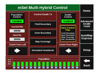
Items on the list that are outlined and in bold are active components of the Swath Control Plan. These components that are active are what the planter will automatically swath on and off to while planting. Those that are not are inactive and will not be controlled to.
