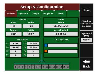
**Step 2:** Ensure that "Planter Make", "Rows", "Spacing", "Active Rows", and "Meter Type" are correct.
