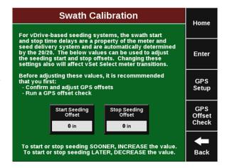
Adjust the Start Seeding Offset to change where the system will begin dropping seeds. Find the distance from where the seeding is actually starting to where it should start by digging. Enter this distance in inches. Negative numbers will move the seeding backwards while positive numbers will more it forwards. Do the same with the Stop Seeding Delay for where the seeding should stop.
