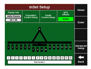
The bottom boxes under the planter indicate the Rate Sections that have been configured and what rows they correspond to.
