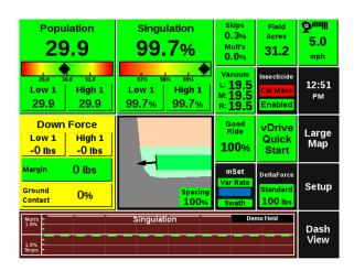
**Note:** The vDrive Quick Start button must be added to the home screen before it can be used. See the 20/20 Operator's Guide for information on configuring the home screen.
